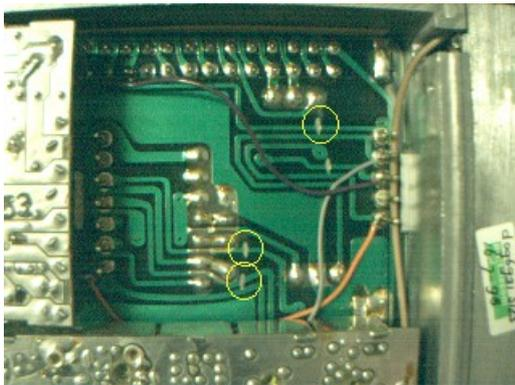
The picture to the left shows the inside of a KF161 from a different production batch. If you have a KF161 like this, then you need to repair 3 PCB traces.
